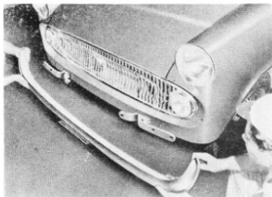
Fig. 10-7 Removing Front Bumper
